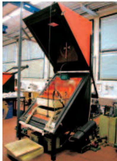
LABORATORIO DI CONDUTTIVITÀ TERMICA: APPARECCHIATURA A TERMOFLUSSIMETRI (PRESSO IL DFT)
